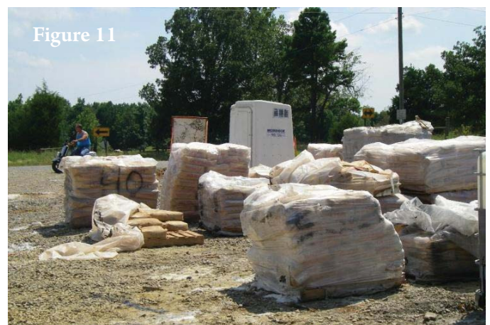
Chemicals stored in this dry chemical area are spilling onto the ground.
